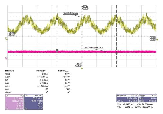
Fig. 13. Experimental results when load is connected to AC Output. Fuel cell current (Channel C1: 2 A/div, 5 ms/div), 48 V-DC Bus voltage (Channel C2: 50 V/div, 5 ms/div).
