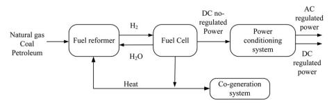
Fig. 2. Fuel cell system basic scheme.
