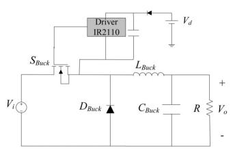
Fig. 8. Bootstrap scheme for Buck converter.
