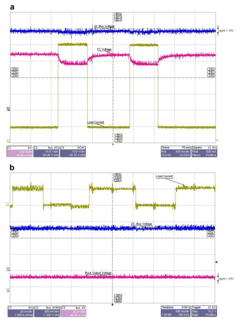
Fig. 12. Experimental results when load is connected to DC links. a) Load connected to Low Voltage DC Bus: Load current (Channel C1: 5 A/div, 500 ms/div), Fuel cell voltage (Channel C2: 10 V/div, 500 ms/div), Low DC Bus voltage (Channel C3: 10 V/div, 500 ms/div). b) Load connected to 12 VDC output: Load current (Channel C1: 20 A/div, 500 ms/div), Buck output voltage (Channel C2: 500 mV/div, 500 ms/div), Low DC Bus voltage (Channel C3: 20 V/div, 500 ms/div).
