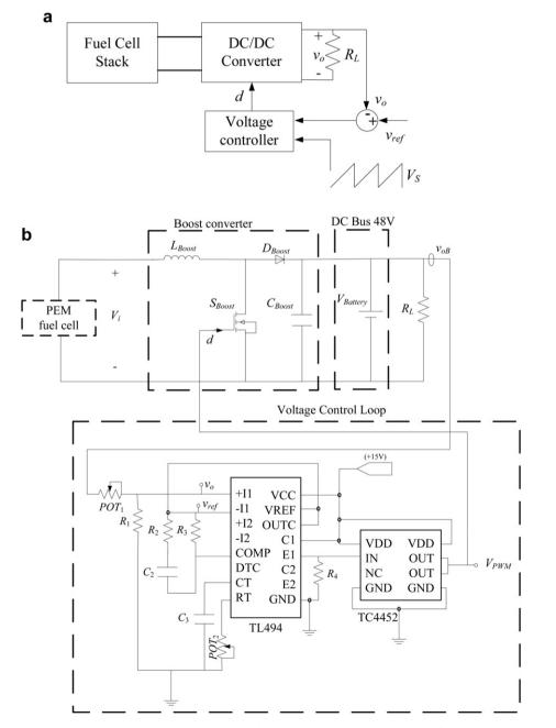
Fig. 7. a: Voltage control loop block diagram. b: Scheme of the voltage control loop applied to PEM fuel cell hybrid system.
