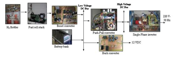
Fig. 10. Simplified scheme with actual systems of the distributed generation system with fuel cell developed.
