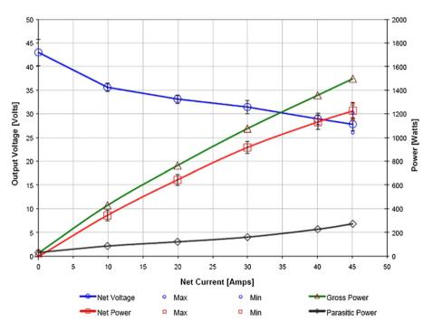
Fig. 6. Polarization and power curves for the Nexa module.
