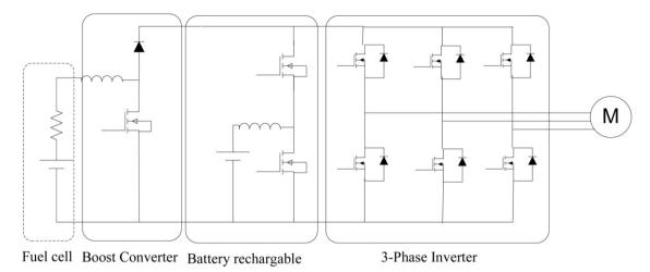
Fig. 5. Circuit topology for a fuel cell hybrid vehicle.
